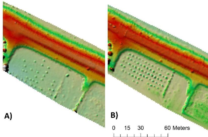
Fig. 6. Digital surface model in resolution of 1 m created from (a) Platform 1: Riegl VUX-1 UAV, (b) Platform 2: YellowScan Mapper.
