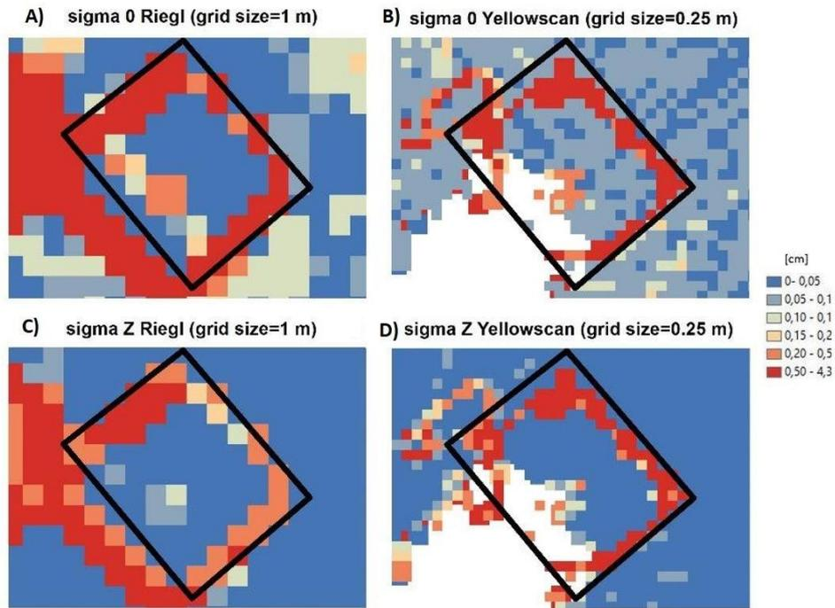
Fig. 9. Differences in distribution of  $\sigma_0$  (a) Platform 1: Riegl VUX-1 UAV, (b) Platform 2: YellowScan Mapper and  $\sigma_Z$  (c) Platform 1: Riegl VUX-1 UAV, (d) Platform 2: YellowScan Mapper values on the roof surfaces.
