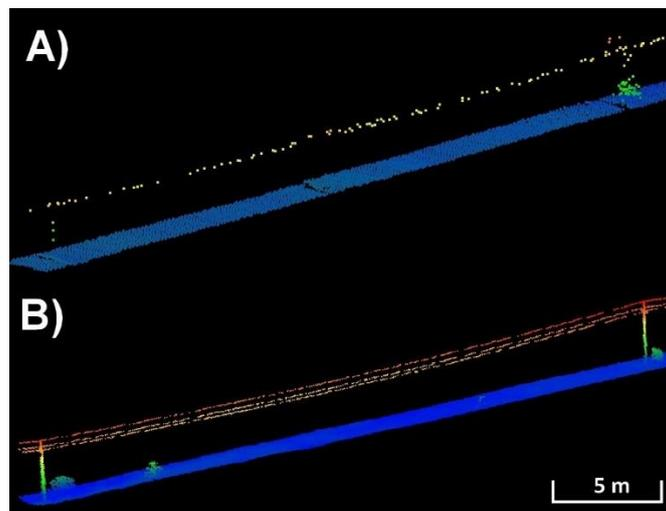
Fig. 8. Example of medium-voltage power line, registered by (a) Platform 1: Riegl VUX-1 UAV, (b) Platform 2: YellowScan Mapper.
