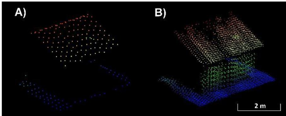
Fig. 7. Point cloud for outbuilding from (a) Platform 1: Riegl VUX-1 UAV, (b) Platform 2: YellowScan Mapper.
