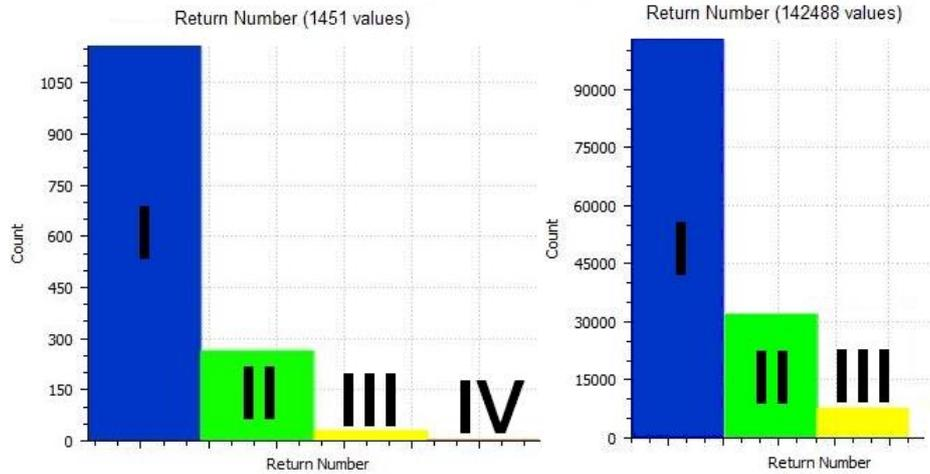
Fig. 11. Histograms presenting point count depending on return number for point cloud registered by: (a) Platform 1: Riegl VUX-1 UAV, (b) Platform 2: YellowScan Mapper.
