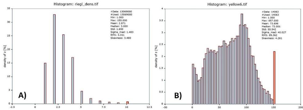
Fig. 3. Histograms presenting point density of datasets acquired with (a) Platform 1: Riegl VUX-1 UAV, (b) Platform 2: YellowScan Mapper.
