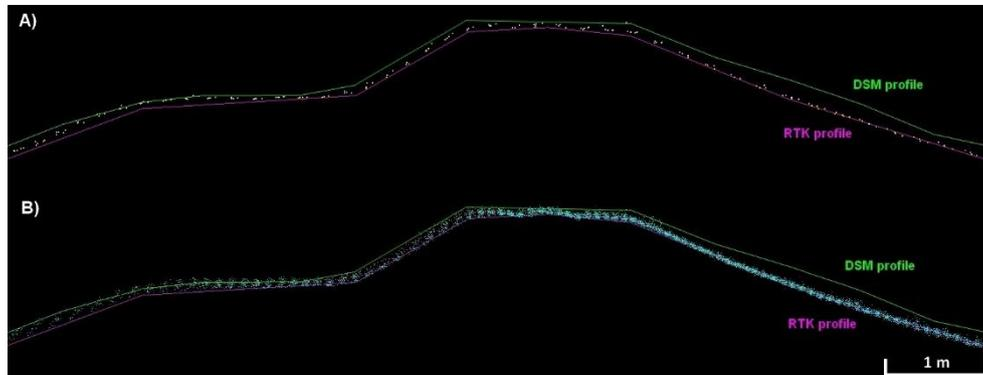
Fig. 12. Cross sections in two variants of the point clouds for (a) Platform 1: Riegl VUX-1 UAV, (b) Platform 2: YellowScan Mapper, together with reference profiles DTM (from RTK) and DSM (from UAV photogrammetry).
