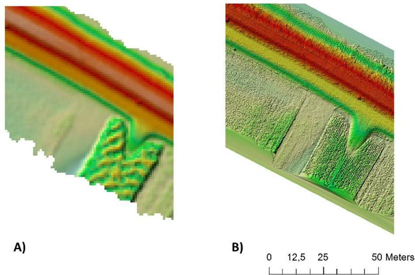
Fig. 5. Digital surface model created from (a) Platform 1: Riegl VUX-1 UAV data with grid resolution of 0.5 m, (b) Platform 2: YellowScan Mapper data with grid resolution of 0.1 m.
