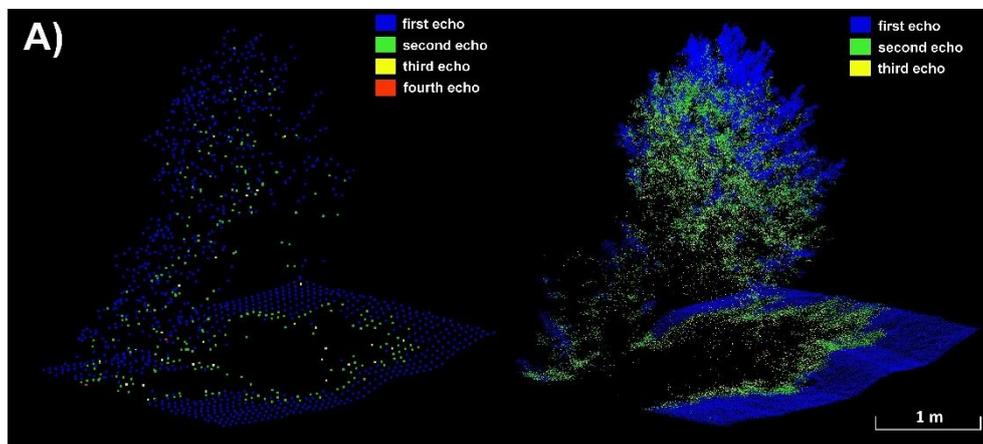
Fig. 10. Visualization of multiple LiDAR returns for a single tree for point cloud registered with: (a) Platform 1: Riegl VUX-1 UAV, (b) Platform 2: YellowScan Mapper.
