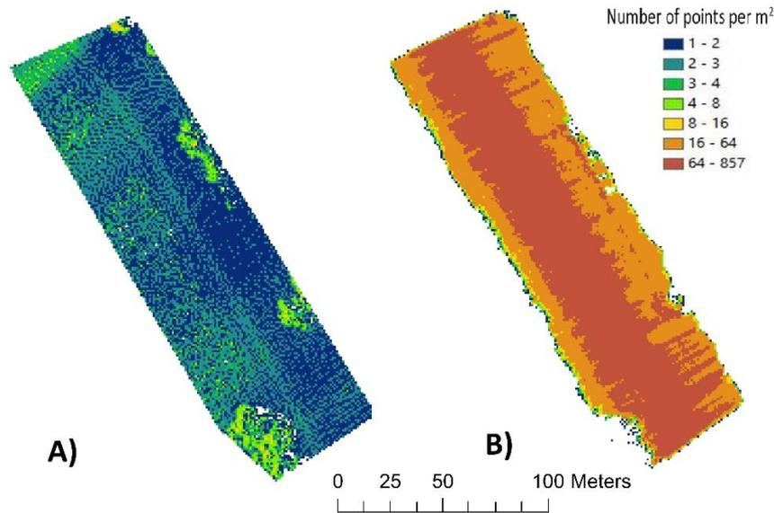
Fig. 4. Raster images presenting point densities: (a) Platform 1: Riegl VUX-1 UAV, (b) Platform 2: YellowScan Mapper.
