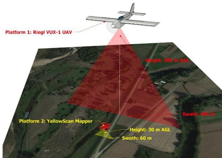
Fig. 1. Graphical comparison of swath width provided with two types of LiDAR sensors from UAV platforms (Platform 1: Riegl VUX-1 UAV, Platform 2: YellowScan Mapper).
