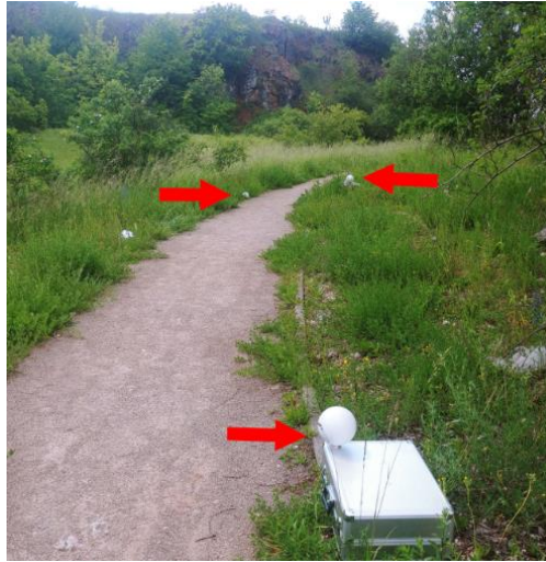
Fig. 7: Spheres used for registration of the TLS scans
