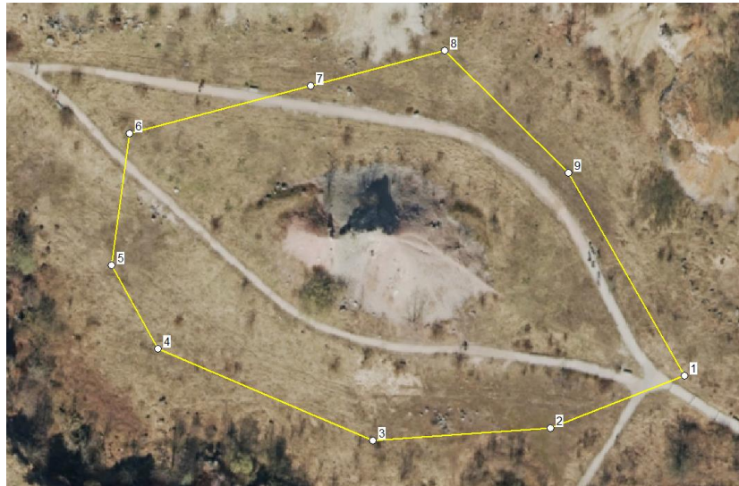
Fig. 4. Sketch of the established survey network (source: own elaboration)
