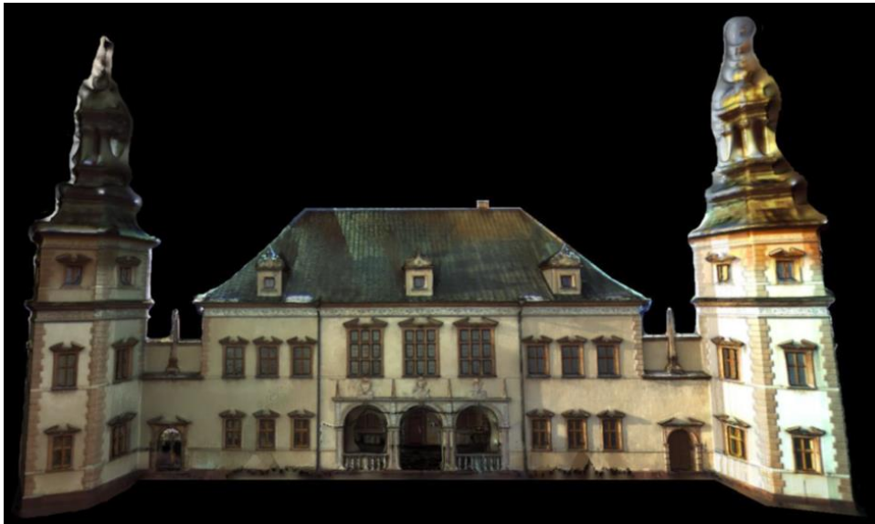
Fig. 13. Laser scanning point cloud with overlaid texture from images ( Cygan & Kania, 2017 )
