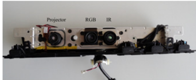
Fig. 7: Disassembled Kinect system
