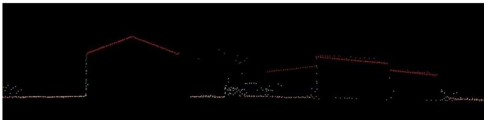
Fig. 11. Classification of overlap points using Terrascan software.
