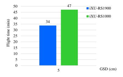
Fig. 3. Flight time for GSD 5 cm
