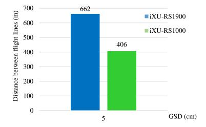
Fig. 2. Distance between flight lines for GSD 5 cm
