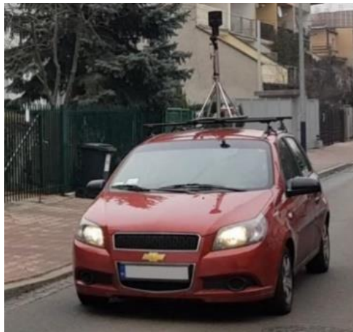
Figure 3 Immersive mobile mapping system placed on the roof of a car. (authors' source)
