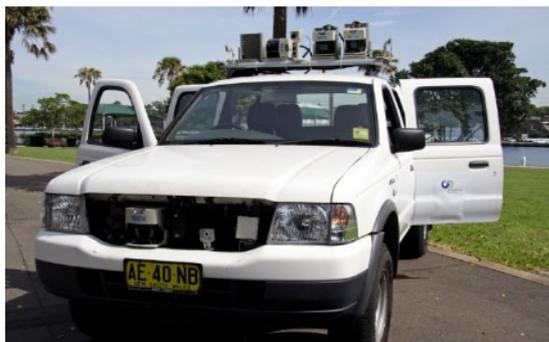
Fig. 5. Multi-sensors mounted on the vehicle
