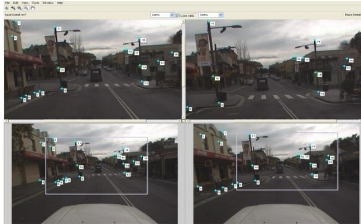
Fig. 9. Measured 18 points on the measurable images selected from the road test.
