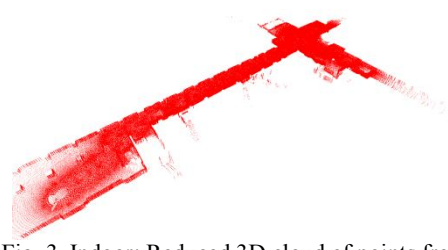
Fig. 3. Indoor: Reduced 3D cloud of points from figure 2 by 3D points above given threshold corresponding to the robot height.
