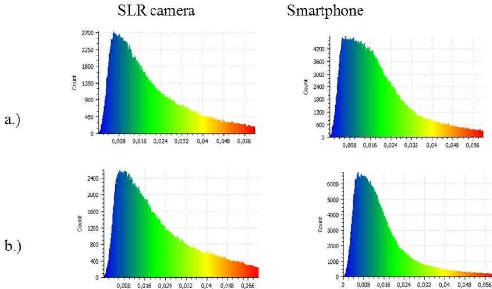
Figure 14. Histograms showing the differences between detail 1, a.) five photos, b.) nine photos; horizontal axis is scaled from 0.000 to 0.060 m.
