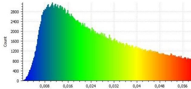
Figure 16. Histogram of difference. Object: wall, number of photos: 22, SLR camera, horizontal axis is scaled from 0.000 to 0.060 m.
