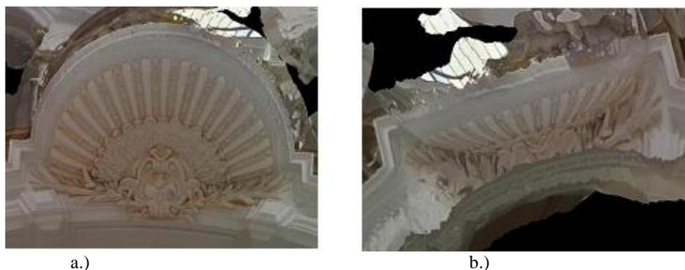
Figure 20. Orthophoto produced with: a.) smartphone and b.) SLR camera.
