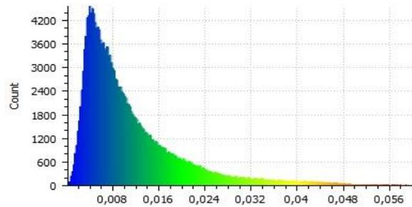
Figure 18. Histogram of difference. Object: detail 2, number of photos: 10, SLR camera, horizontal axis is scaled as above from 0.000 to 0.060 m.
