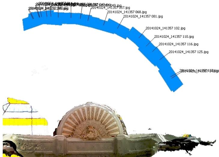
Figure 5. Camera positions for the selected frames: detail 1, view from the bottom.
