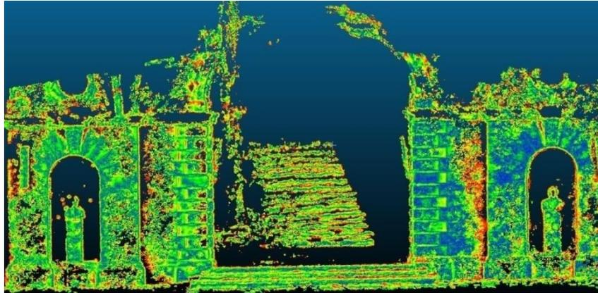
Figure 15. Object: wall, number of photos: 22, SLR camera
