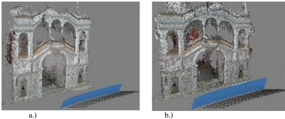
Figure 19. Models produced with a.) medium and b.) high point densities.
