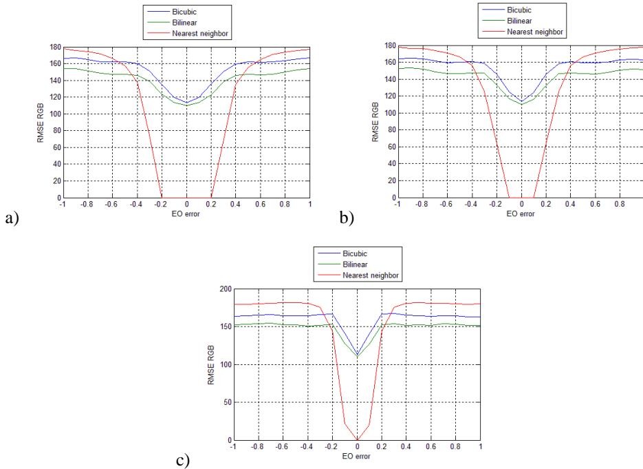
Fig. 11. Effect of EO on colorization accuracy for synthetic data: a) errors of linear EO, b) errors of angular EO, c) errors of linear and angular EO.
