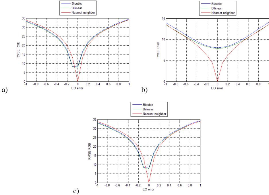
Fig. 12. Effects of EO on colorization accuracy for natural data: a) errors of linear EO, b) errors of angular EO, c) errors of both linear and angular EO.
