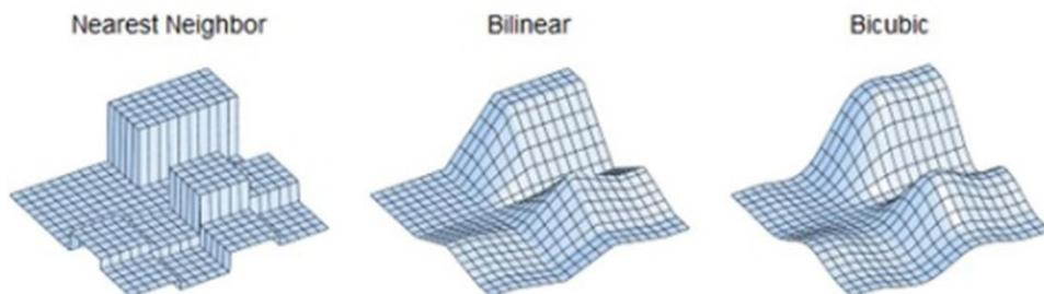
Fig. 2. Interpolation methods applied as part of the colorization algorithm (Getreuer, 2011).
