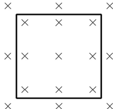
Fig. 4. Distribution of 17 test points in the synthetic cloud with a square pixel range
