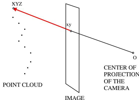
Fig. 1. Geometry of point cloud colorization (Rzonca, 2013).
