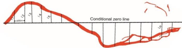
Fig. 7. Position of conditional “zero line” and perpendiculars
