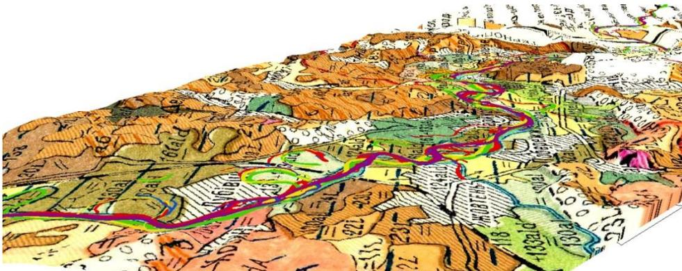
Fig. 9. First section of riverbed and soil map overlaid on DTM
