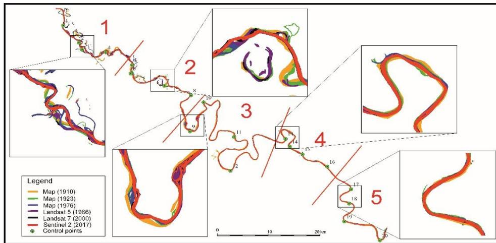
Fig. 5. Common view of Dniester riverbed digitized on topographical maps and satellite images at different epochs.
