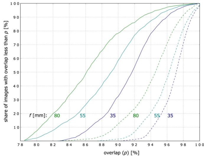
Fig. 7. Empirical cumulative distribution functions of the percentage of the planned area covered by photographs. The continuous lines: the stabilizing system turned off. The dashed lines: the stabilizing system turned on. The simulation was performed for three different focal length values and used the medium-format camera Phase One iXA 180.
