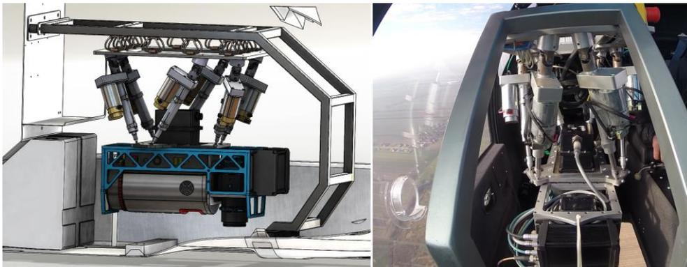
Fig. 2. The system prototype CAD model (to the left); the system photographed in flight (to the right) (Kolecki *et al.*, 2016)
