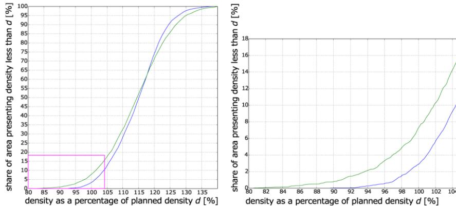
Fig. 5. Empirical cumulative density distribution functions of points in a cloud, expressed as a percentage of the planned density. In green: the stabilizing system turned off. In blue: the stabilizing system turned on. To the right: the zoomed area of the diagram, marked by a rectangle.
