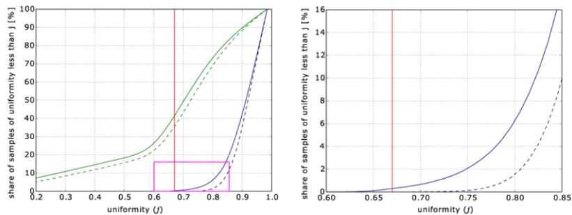
Fig. 6. Empirical cumulative uniformity distribution functions. The dashed line: the stabilizing system turned on. The continuous line: the stabilizing system turned off. In blue: filtered data. In green: raw data. To the right: the zoomed fragment, marked by a rectangle. The red vertical line marks the threshold value for the ISOK project, equal to  $2/3$ .
