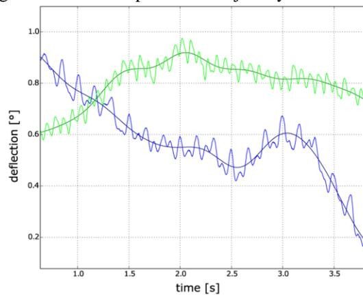
Fig. 4. Deflections of the  $roll$  (blue) and  $pitch$  (green) components over time - an example. Raw and filtered data are presented.
