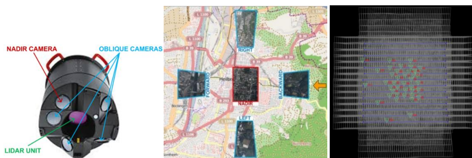
Figure 1. The Heilbronn CityMapper dataset. Left: the Leica hybrid sensor. Centre: the planned flight trajectories (blue lines), image footprints (white polygons) and control points (green triangles). Right: the image footprint of one single exposure (nadir image in red, oblique images in blue).
